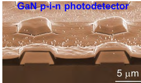
Fig. 3 Cross-section SEM of a core/shell/shell p-i-n pillar array
