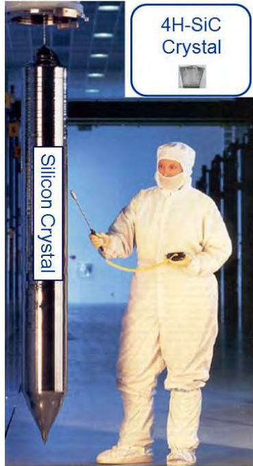
Fig. 1: Pictorial representation of a silicon wafer ingot grown by the Czochralski method [3] and SiC wafer grown by sublimation growth using the modified Lely process [2].
